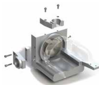
Fig. 5: Thermo Scientific ES071 source with mounting kit (exploded view)
