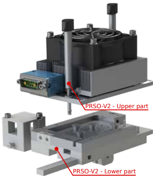
Fig. 1: Upper and lower part with column pins
